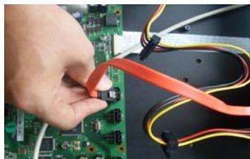
5. Use the special data cable to connect the HDD and the SATA port
