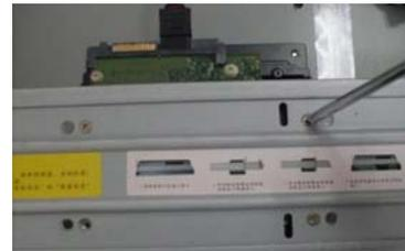
3. Use four screws to fix HDD.
