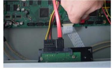
9. Use the special data cable to connect the HDD and the SATA port. Close the chassis and fix the screws to secure firmly.
