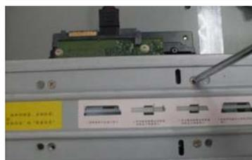
5. Use four screws to fix HDD.
