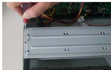
2. Remove the HDD upper bracket
