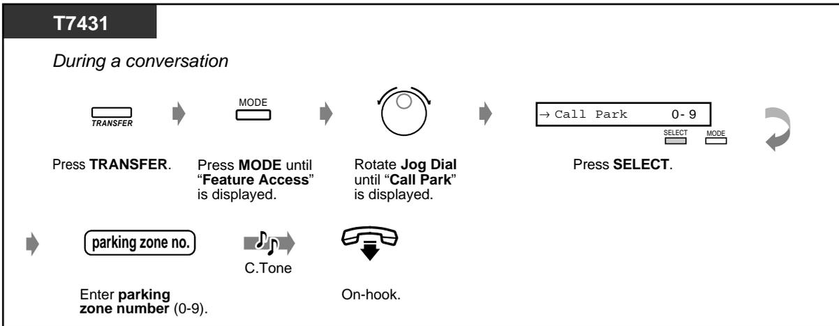
Press **TRANSFER**.      Press **MODE** until "Feature Access" is displayed.      Rotate **Jog Dial** until "Call Park" is displayed.      Press **SELECT**.      Enter **parking zone number** (0-9).      C.Tone      On-hook.
