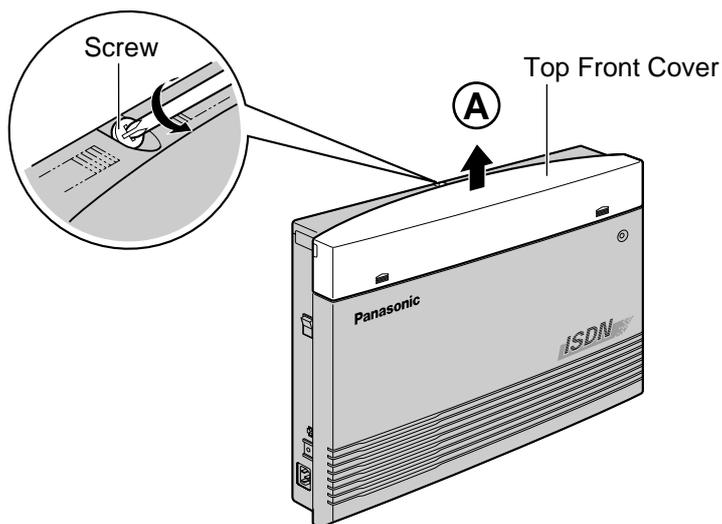
3. Loosen the 2 screws of the both sides of the unit.
