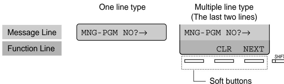
The message line guides you through programming and lets you confirm your selection. For example, when "Jack No? ->" is displayed, enter the jack number. The display shows up to 16 characters at a time. To scroll the display, press -> or <-. The function line shows you the function of the Soft button located below it. When the SHIFT button light beside the display is on, subtitles are available. Press the SHIFT button to confirm the available functions.
